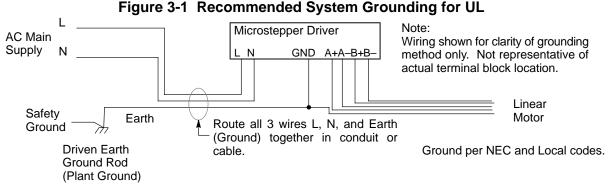
Note: Use shielded cable for driver signal wires. Route driver signal wires in conduit. These wires must be kept separate from power and motor wires.
